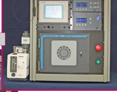
SCE-108 Shown with RF Matching Network Multi-Process PLC Mass Flow Controls
